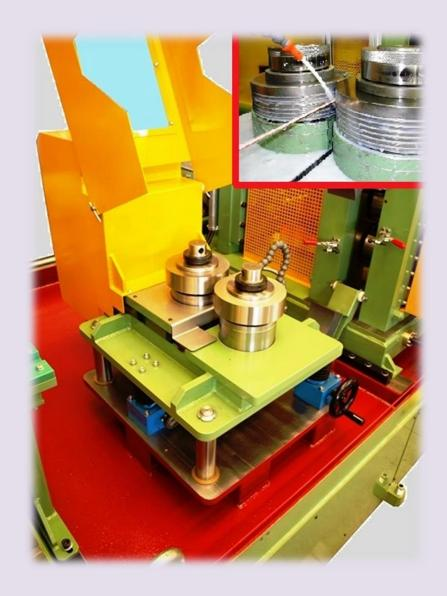
Translation system rolling mills cages to use the entire surface of the rollers without losing the machine axis.
