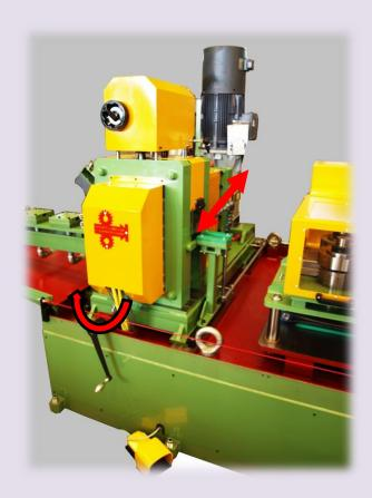
Cleaning flat wire and rolls system with blowers, turbofan and felt.
