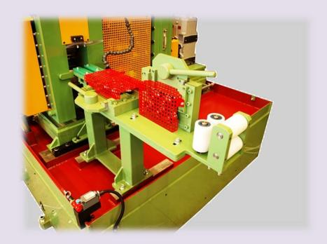
**No. 1** - Rolling mill machine at 3 rolling cages with cylinders of diameter 240-180-180 mm and working band of 100mm.
