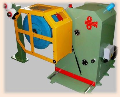
Independent Traversed take- up suitable for insulated machines, realized in order to wrap the wire conductors of rectangular section (flat wire). The reel is supported by a motorized oscillating arm able to unload the reels on the floor without the use of lifting equipments.
