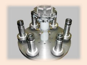
**Tangential** insulating head suitable for insulated yarn. The tape tension is performed by a self-regulating system of springs. The head is equipped with a tape broken alarm system and an alert system of end tape.
