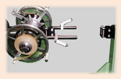
Tangential taping head suitable for insulating tape. The tape tension is performed by a self-regulating system of springs. The head is equipped with a tape broken alarm system and an alert system of end tape.
