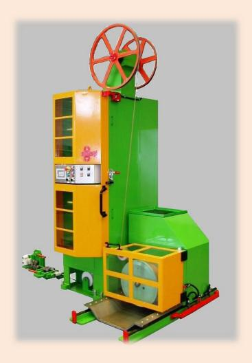
Vertical taping line suitable for insulation of conductors with a rectangular section (flat wire) completely modular. On this machine may be installed 3 types of insulation heads (tangential head, concentric head, head for yarn), and these are replaced in few minutes.
