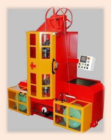
Vertical taping line suitable for insulated conductors with round section (wire- strand conductor) completely modular. On this machine may be installed 3 types of insulation heads (tangential head, concentric head, head for yarn), and these are replaced in few minutes.
