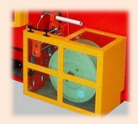
Take-up placed inside the insulated machines realized in order to wrap the wire conductors of round section (wire – rope) by traversing system motorized in C.A.
