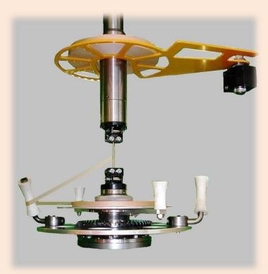
Concentric taping head suitable for insulating tape. The tape tension is performed by a selfregulating system of springs. The head is equipped with a tape broken alarm system and an alert system of end tape.
