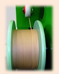
Traversed take- up placed inside the insulated machines realized in order to wrap the wire conductors of rectangular section (flat wire) by traversing system and a specific platform in order to load & unload the reel.
