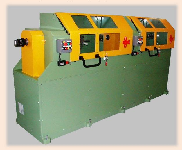
Horizontal taping machine suitable for insulation of conductors with a rectangular and round section (flat wire- wire- strand conductor)
