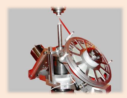
The tape tension is performed by a selfregulating system of springs. The head is equipped with a tape broken alarm system and an alert system of end tape.
