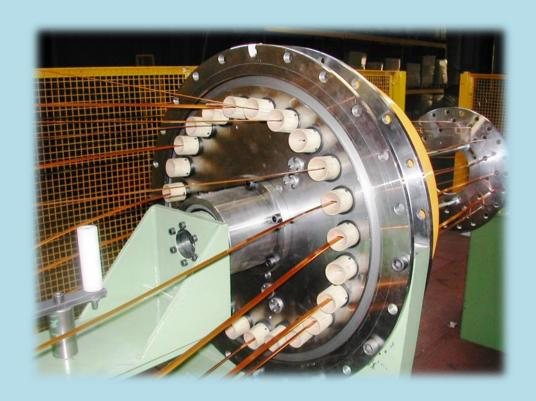
The transposition will be effected through an Arens transposing head thanks a sophisticated system of levers but easy to adjust.
