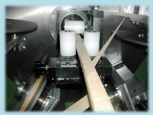
The dragging of the transposed conductor will be effected by a drawing type "Caterpillar" composed of rubber straps with adjustable closing pressure.
