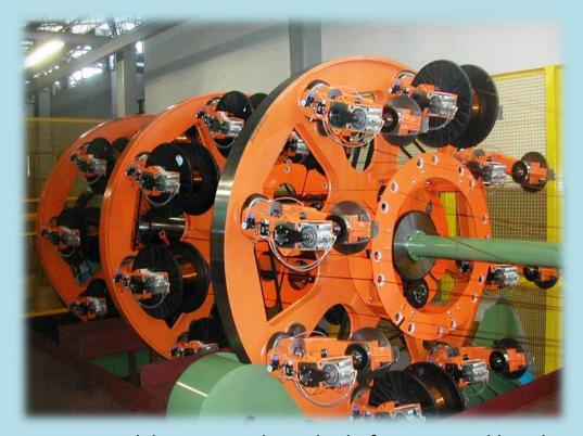
The disks are connected by a central sturdy shaft supported by a bearing in the back position. In the front part and in the central part of the cage the discs are supported by a roller system in Gesadur anti-wear.
