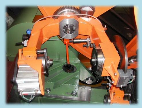
In order to ensure the parallelism and maintain the proper arrangement the flats wire are moved by a mechanical stranding machine that it is mechanically connected to the rotation of the unwinding cage.
