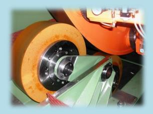
The coils cradles are completed of an independent braking system. If the customer needs it can be composed by a disc and pneumatic tailstock or regular strip with ferodo.
