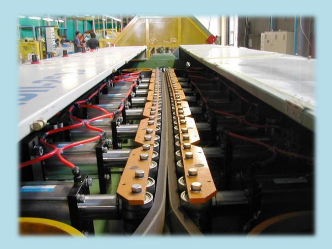
At the end of this process the insulated and transposed conductors will be winding through a take-up portal in order to receive a wide range of coils. During the winding process the coil is made to translate in such a way as to be able to wind the conductor in "turn-turn" and throught a special equipment it is controlled the isolation of each flat wire.
